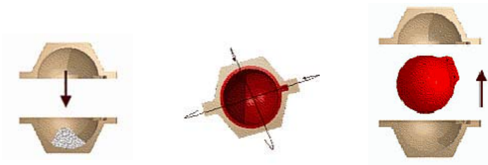
LOADING RESIN INTO THE MOLD
